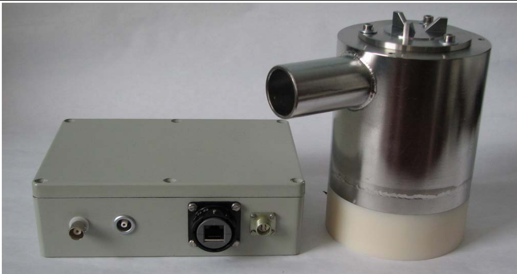
General view of the ULSE and its electronic box.
