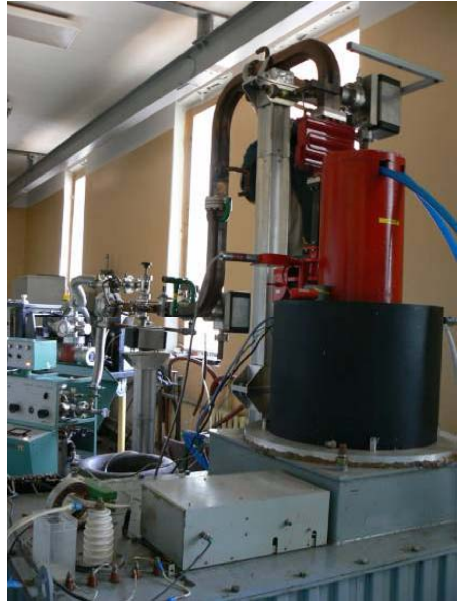
RF test bench on the base of operational klystron "Thompson TH 2129".
