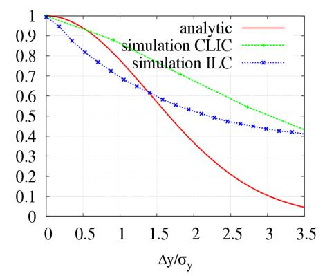
Vertical separation between beams  $\Delta y$  mainly from fast ground motion, and damping ring extraction errors
