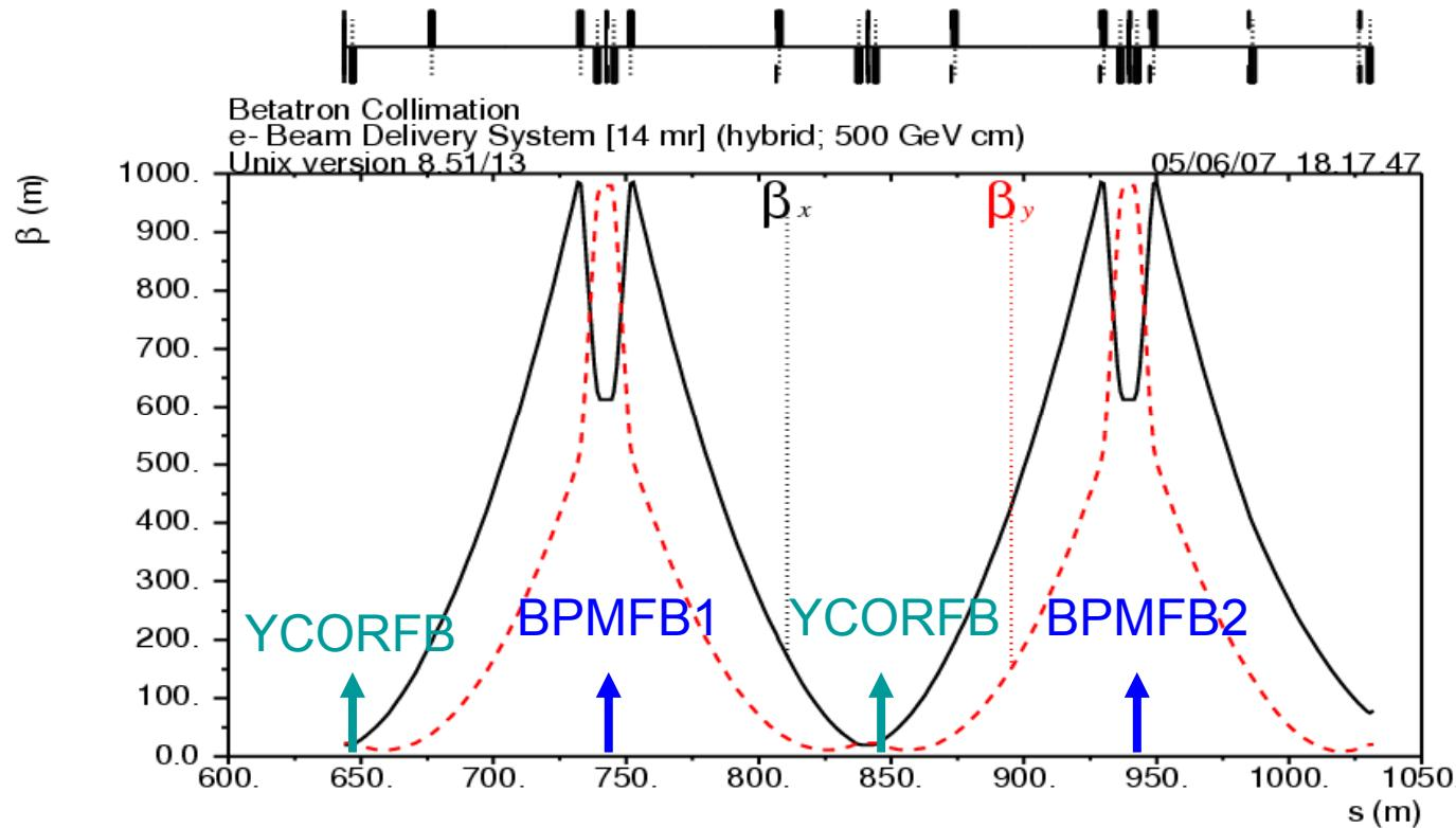
Pair of kicker-BPM for orbit correction in both vertical degrees of freedom (y-y')
