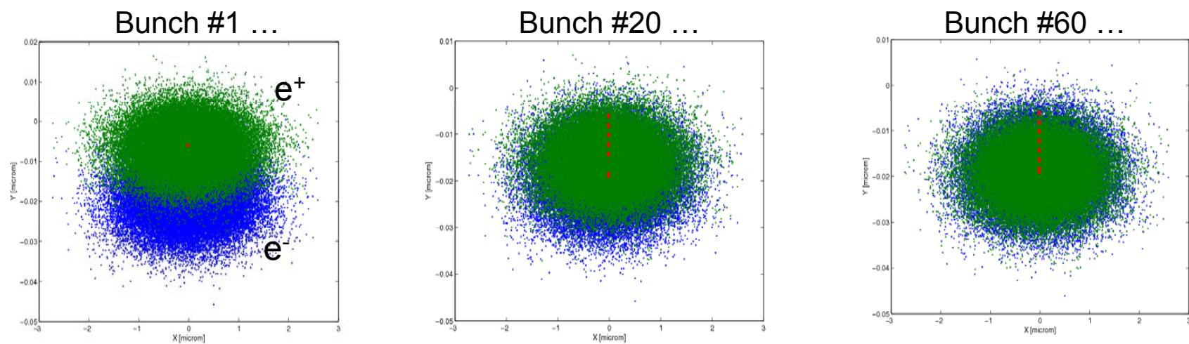
Example of transverse profile evolution at the IP with FB system switched on
