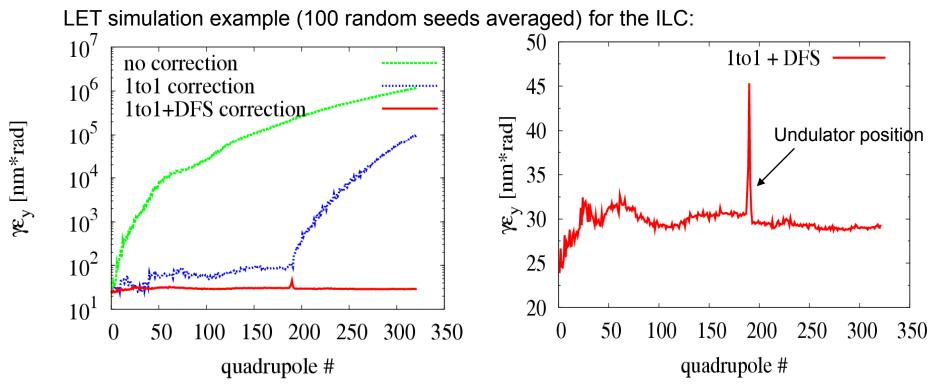
Undulator alignment being studied by Duncan Scott et al. (Daresbury). In this simulation we have replaced the undulator by a matching transport matrix ! December 11-13, 2007 Javier Resta Lopez 5
