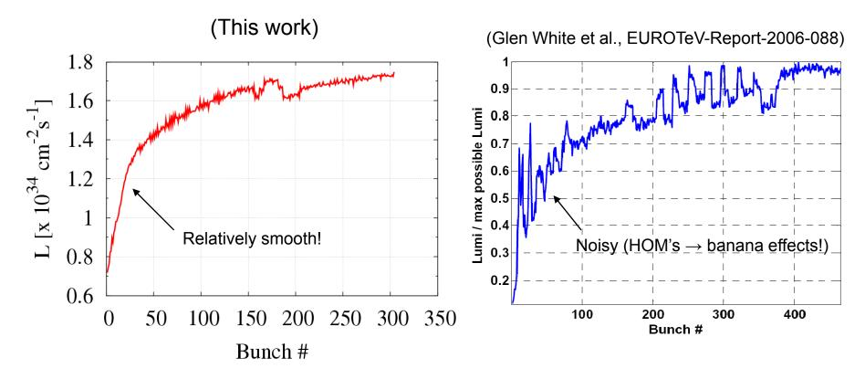
Assuming a pessimistic case of 40 % emittance growth in the linac Applying 0.2 s of GM model C to the Linac + BDS (1 single seed) Additional component jitter: 25 nm for the quads in the BDS; 50 nm for the quads in the Linac
