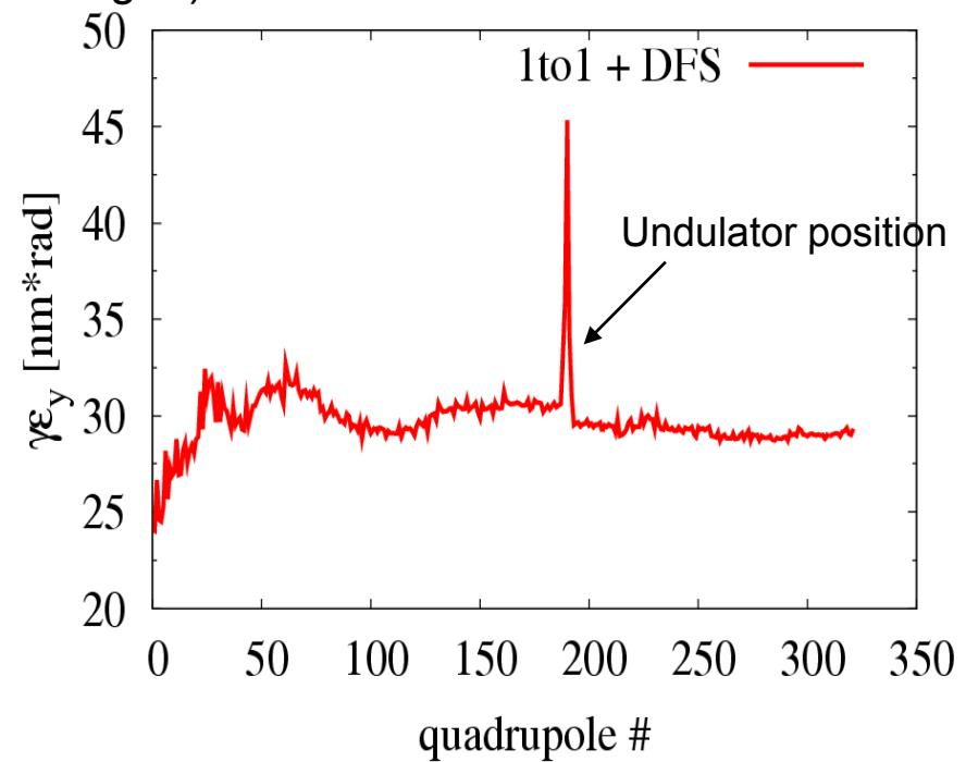
Undulator alignment being studied by Duncan Scott et al. (Daresbury). In this simulation we have replaced the undulator by a matching transport matrix !
