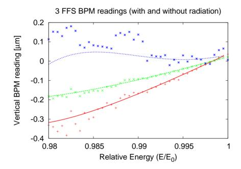
$\Rightarrow$  We decided to calculate the response matrix R neglecting the synchrotron radiation emission
