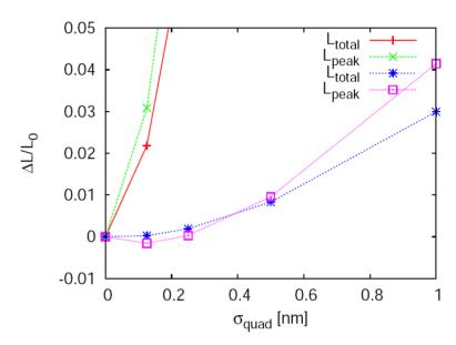
$\Rightarrow$  stability of 0.5 nm for quadrupoles and 0.1 nm for final doublet quadrupoles
