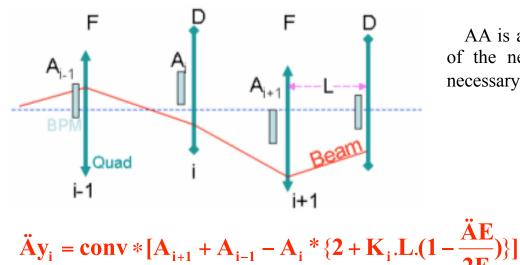
AA is a local method in which the BPM readings  $(A_i)$  of the neighbouring quads are used to determine the necessary shifting of a central quad  $(y_i)$ .
