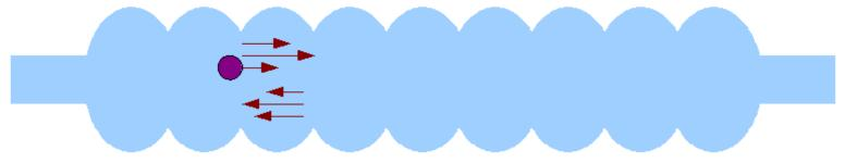
Dipole mode: Amplitude proportional to bunch transverse position Phase determined by bunch arrival time for position offset
