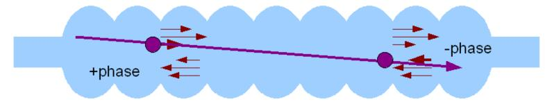
Beam at an angle will excite dipole mode with 90 degree phase shift relative to signal from position offset Amplitude proportional to angle X effective mode length (~ Meter)
