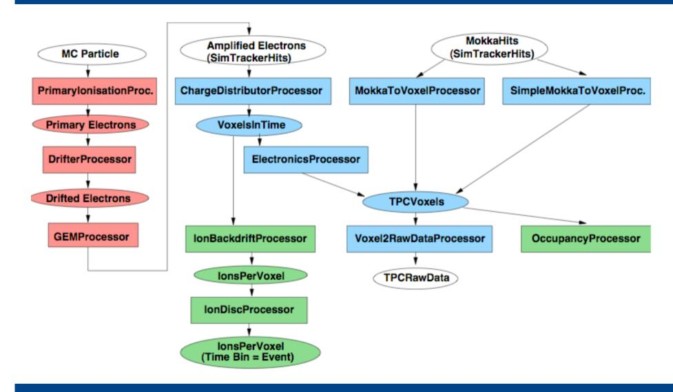
The pads are sampled with a given frequency, which results in a 3D binning of the TPC (voxels).
