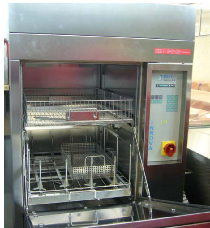
Industrial washing / drying machine (Used at DESY for cleaning of UHV parts )
