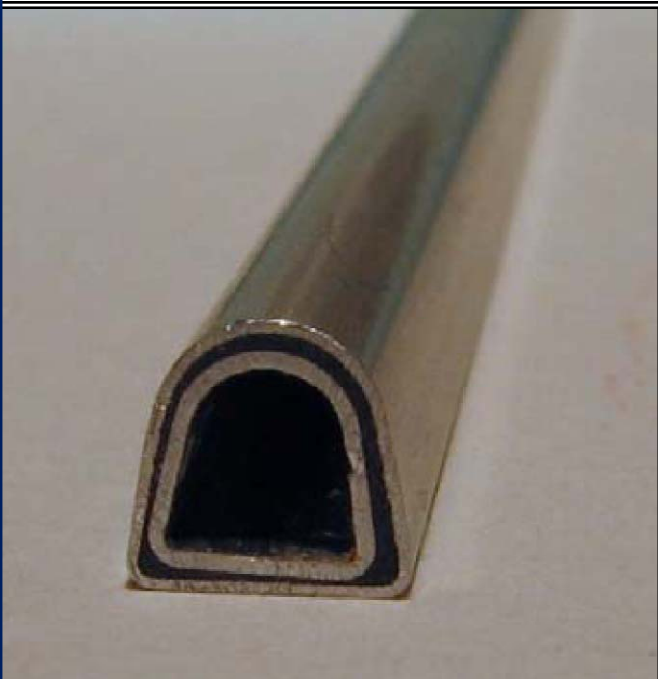
View of the section of the “inserted” pipe. Note the excellent coverage of the thermal compound
