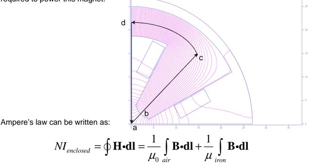
The last integral in iron can be ignored because the permeability of iron is quite large. Similarly, the portion of the integral between points d and a will be zero due to symmetry (ie, the magnetic field lines are perpendicular to the path of integration). Thus we only need to evaluate the integral between points a and b.
