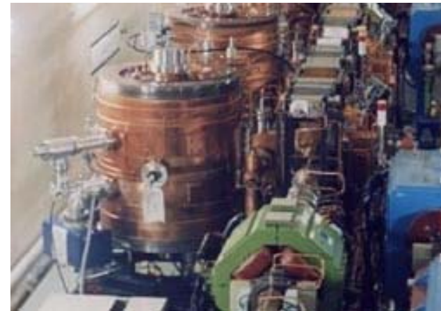
ARES for KEKB with storage cavity for beam stability
