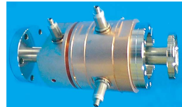
Cavity BPMs, for use with Q magnets with 100nm resolution (PAL, SLAC, KEK)
