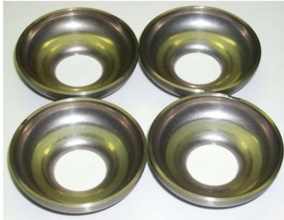
Disks are then deep drawn in a hydraulic press
