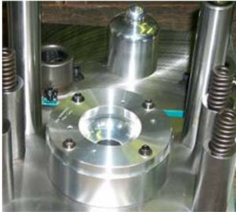
Disks are then deep drawn in a hydraulic press
