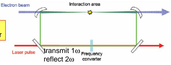
Pulse Stacking Cavity
