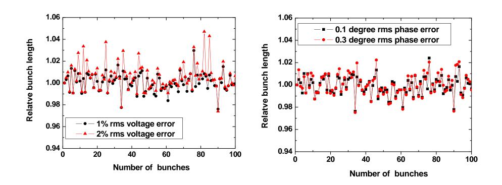
100 successive bunches due to rf voltage jitter (left) and rf phase angle jitter (right).
