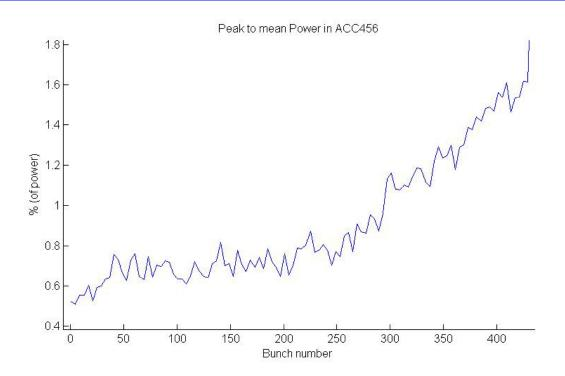
Peak to mean difference of total forward power measured using the sum of all forward power probes in ACC456 cavities adjusted by a square law coeff.
