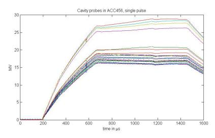
Power probes in ACC456 cavities are not calibrated. Cavity Qs are close to each other. If calibrated there should be a quadratic relationship between power and voltages. So, I normalized power levels to voltage levels using a quadratic law.
