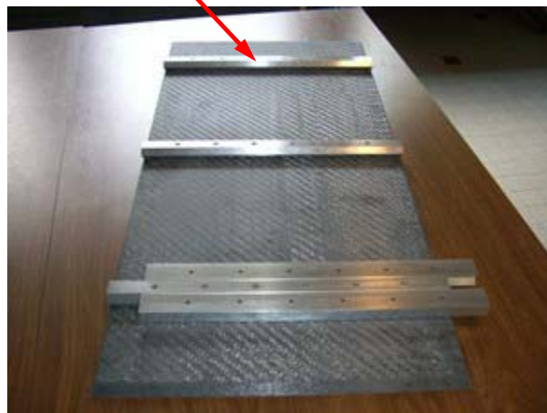
EUDET 15mm thick plate with it's rails; ready to be assembled with alveoli layers
