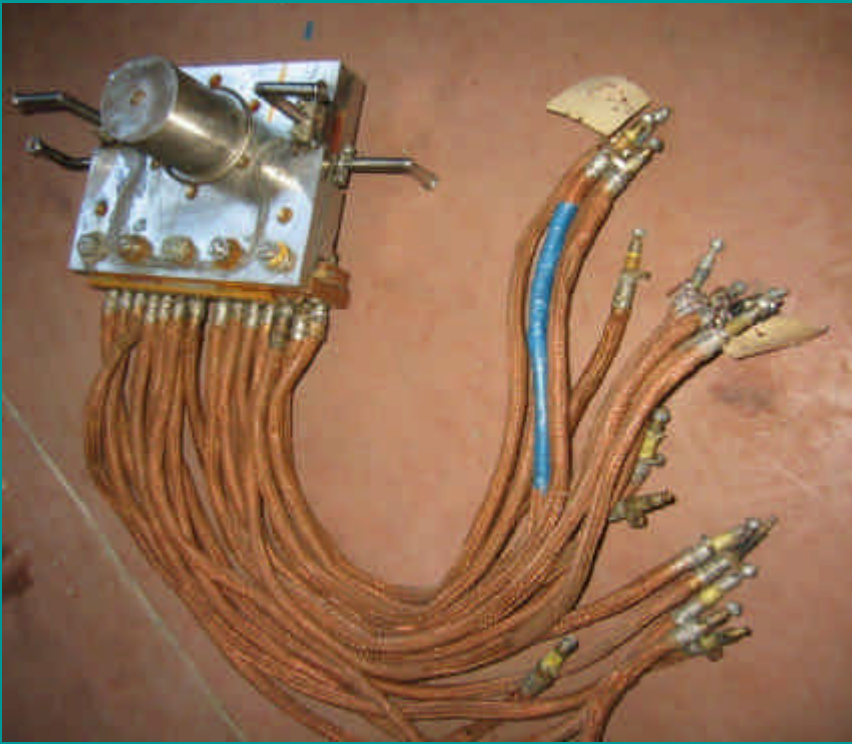
Lithium lens with feeding cables connecting lens with secondary windings of a transformer. (Courtesy of Yu. Shatunov, BINP).
