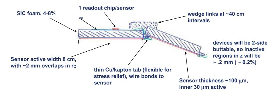
\*\* single layer Cu/kapton stripline runs length of ladder, double layer in region of tabs (~5 mm wide) which contact each sensor. Single Cu/kapton stripline runs round the end of each barrel, servicing all ladders of that barrel
