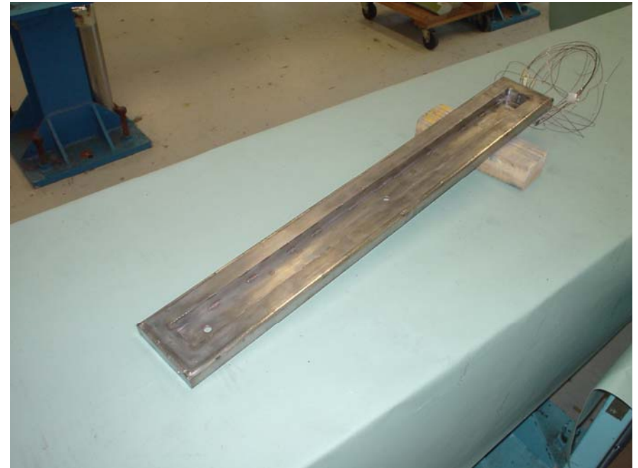
SC Coil after collar welding and epoxy impregnation (ready to install)
