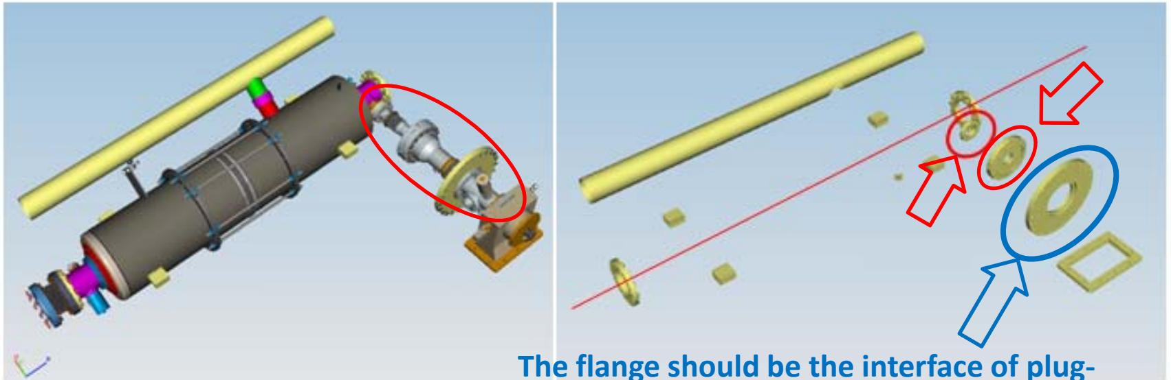
The flange should be the interface of plug-compatibility.
