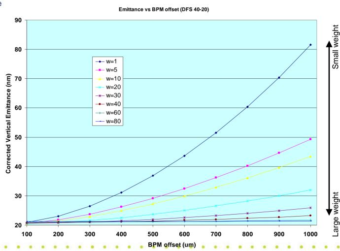
Corrected Emittance= Energy Correlation numerically removed.
