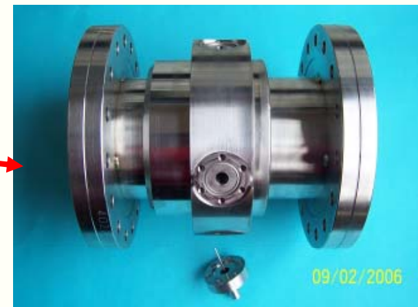
Re-entrant cavity BPM installed in a warm section on the FLASH linac
