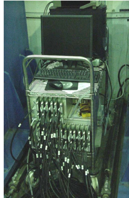
National Instruments SCXI data acquisition system and Labview software, shared with 1-cell thermometry system
