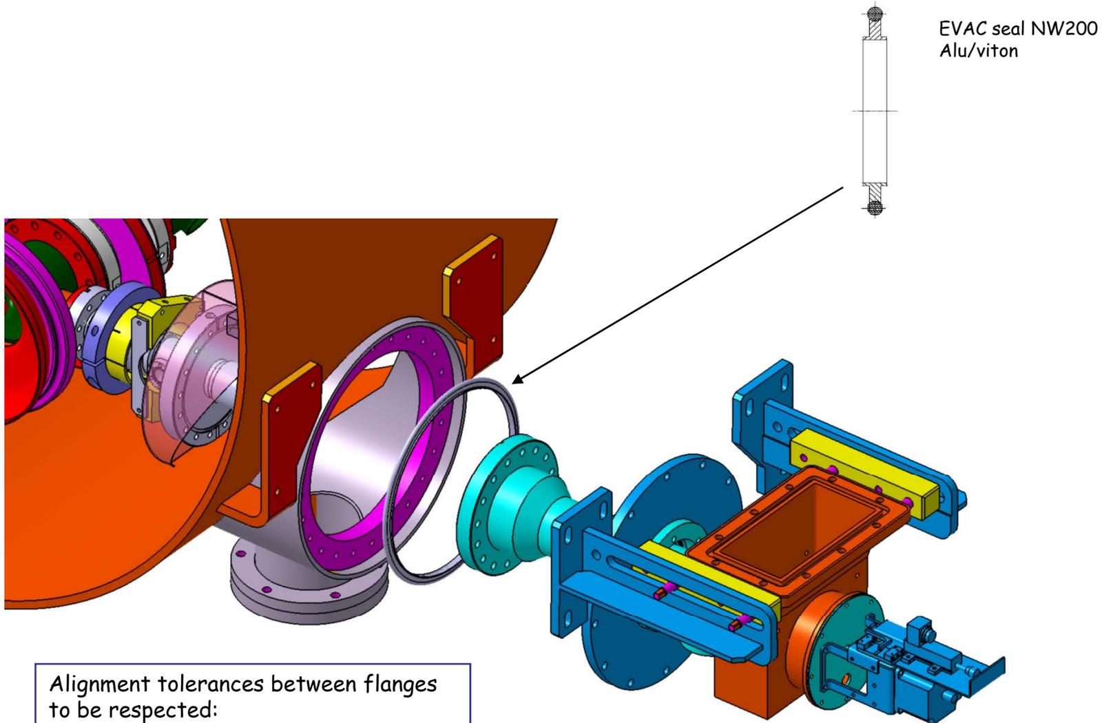
Alignment tolerances between flanges
