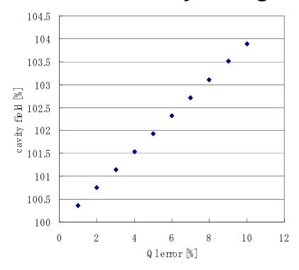
■ If the 6% field increase (+2MV/m) will not acceptable, external QI control system by such as 3-stub should be installed.
