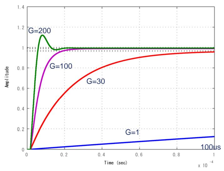
Faster response at high gain *(but larger drive will be necessary)*. Fast FB needs larger driving power.
