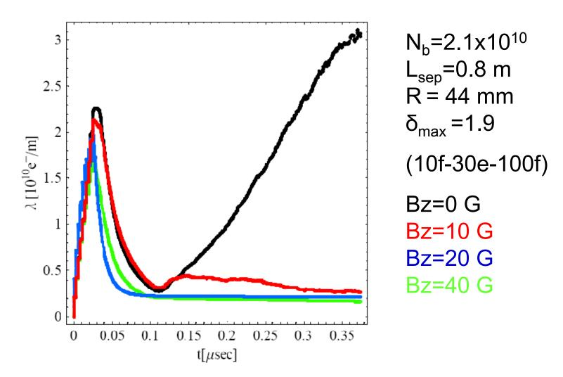
Photoelecrons are produced only during the passage of the first 10 bunches.
