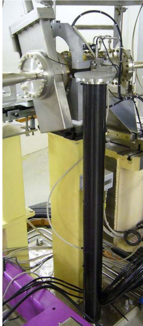
Reference pillar supporting linear encoders
