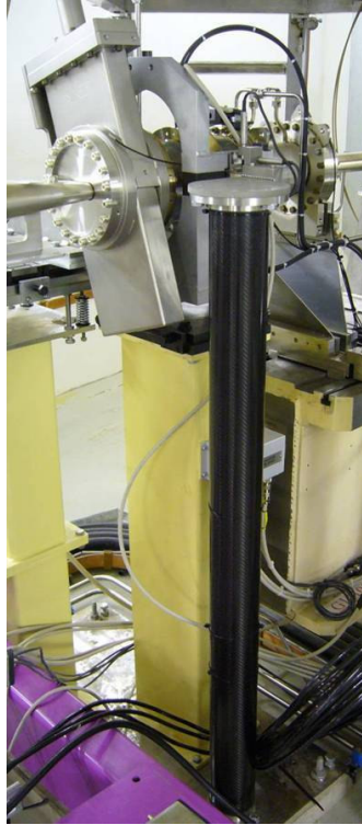
Reference pillar supporting linear encoders
