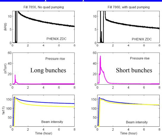
Short bunches with same intensity lead to smaller luminosity.
