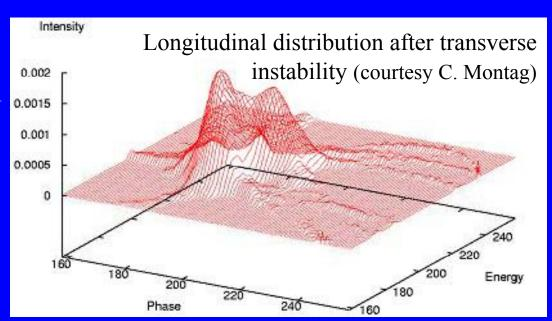
→ Electron clouds can lower stability threshold, will gain more operational experience in current Au-Au run
