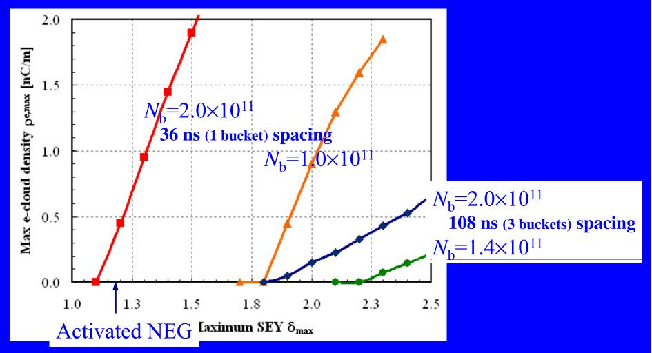
Expect serious e-cloud problems for  $N_b$ =2.0×10<sup>11</sup> and 36 ns bunch spacing (Analysis needed for warm double beam, and cold regions also.)
