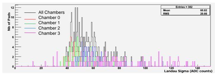
12x32 pads MicroMegas shows a larger sigma disparity
