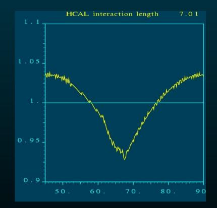
The space between calorimeter and coil is too small in Mokka, the mean interaction length is similar to the analogue case
