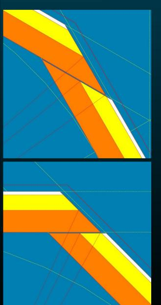
The total thickness of Ecal is 185 mm including today a back plate of 15mm We consider leaving 30mm between Ecal and Hcal for rails and support, cooling, power, signal
