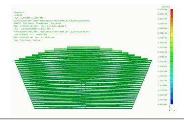
Module standing Maximum deformation: 0.6 mm
