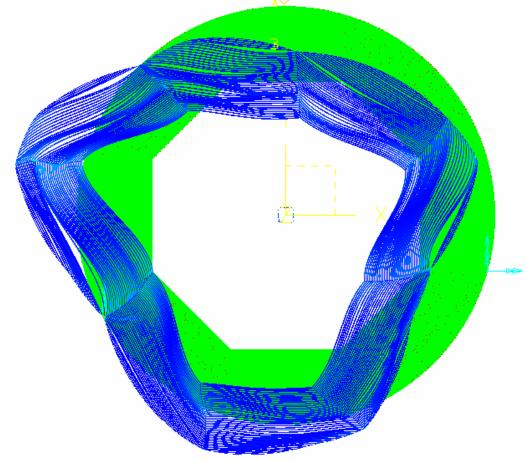
Maximum deformation: 10.4 mm Maximum stress (von Mises): 158 N/mm<sup>2</sup>
