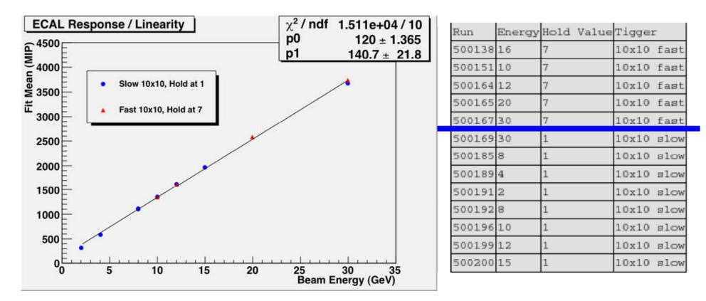
linearity in slow and fast trigger mode looks good... noise still to be checked same calibration applied to both data sets
