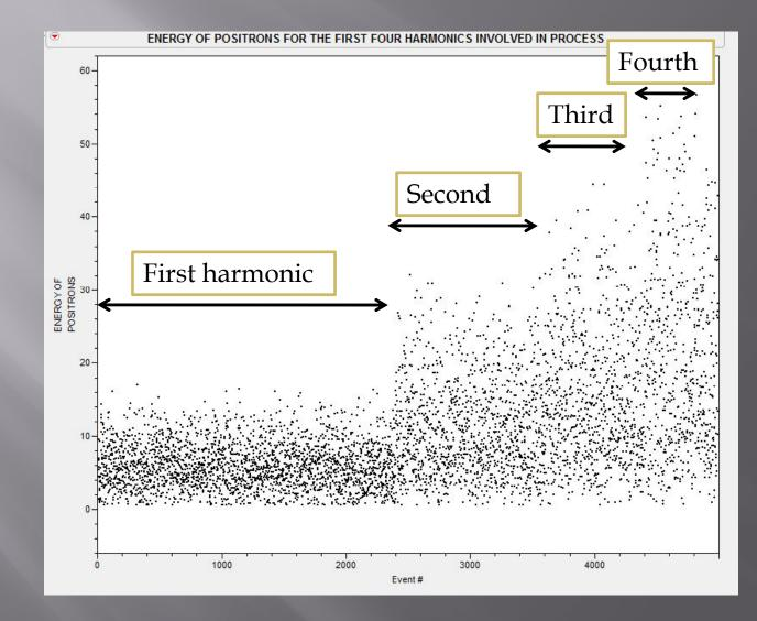
Example: energy for each particle generated by 1-4<sup>th</sup> harmonics of Undulator
