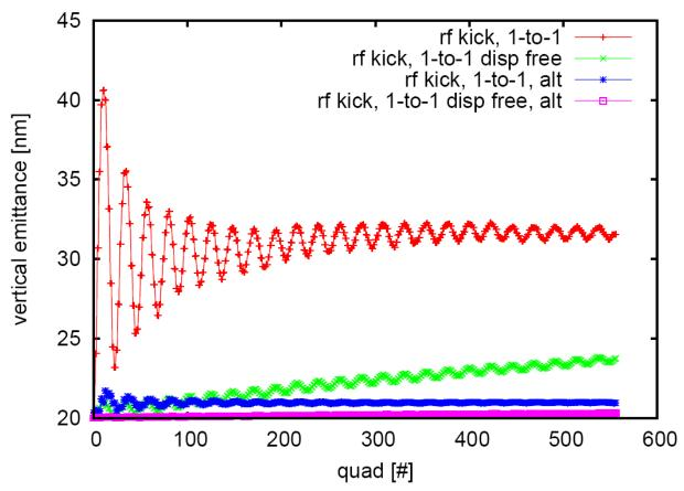
• "alternate" reduces the RF-Kick and allows to use the "new" configuration, that compensates the wakes.
