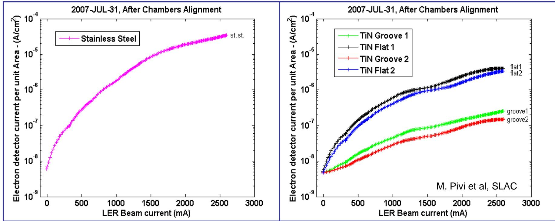
Electron cloud signal in stainless steel chamber.
