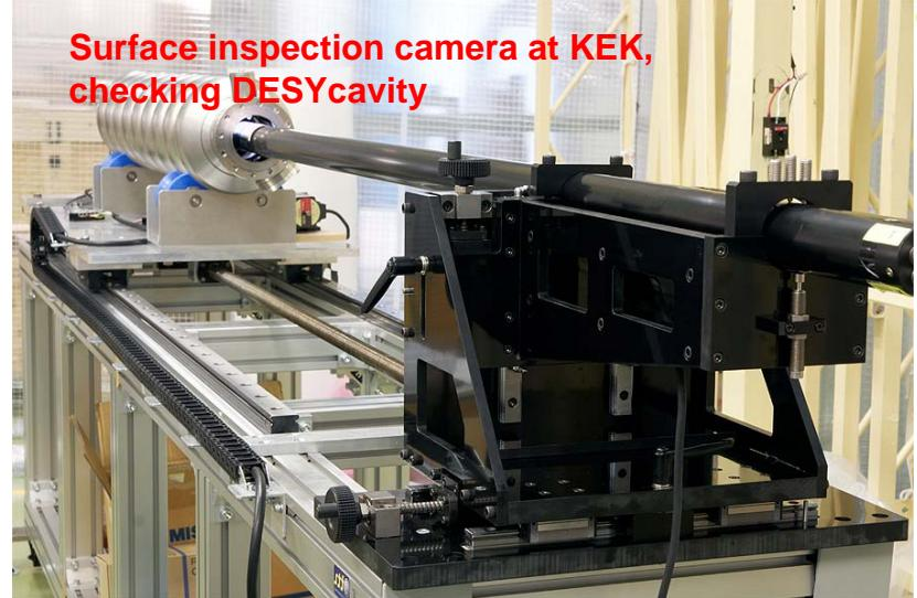
Surface inspection camera at KEK, checking DESY cavity
