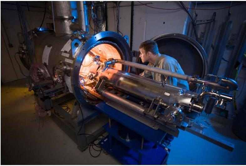
9-cell cavity near vertical test stand
