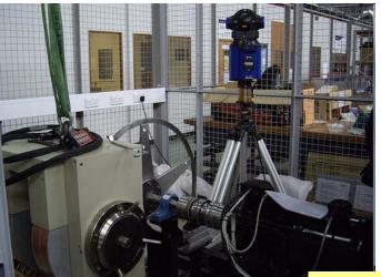
Target Wheel Installation and Testing at low RPM
