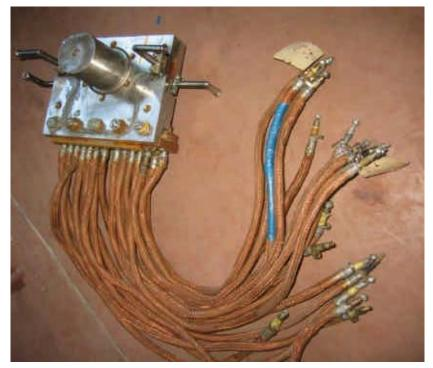
Lithium Lens with feeding cables. (Courtesy of Yu. Shatunov, BINP)
