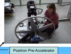
Target Station incl. DL Target Wheel and Positron Capture
