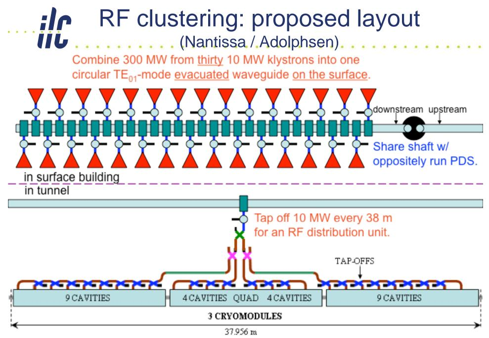
With extra transmission loss, feeds ~27 RF units = 1.026 km. (shaft serves 2.052 km)
