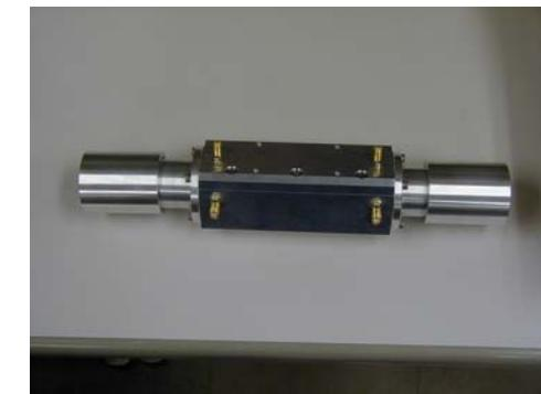
Al connection tube with finger-contactor
