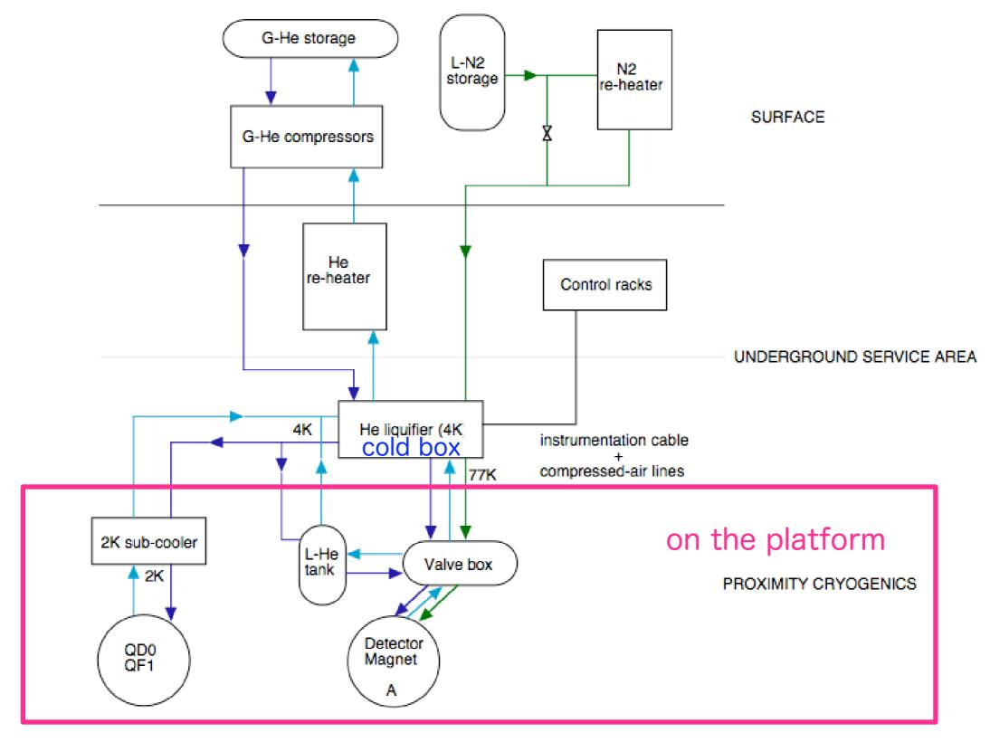
Comment: Separate cryogenics systems for the detector magnet and the final focus magnets should be considered for easy/simple handling.
