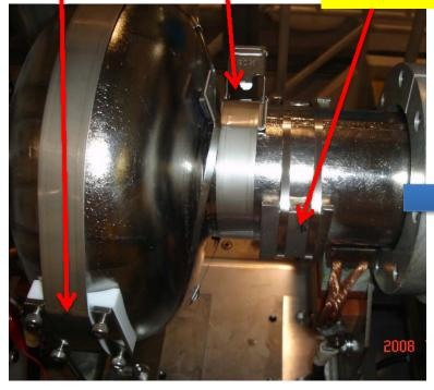
6 Nb samples were dressed on the special cavity
