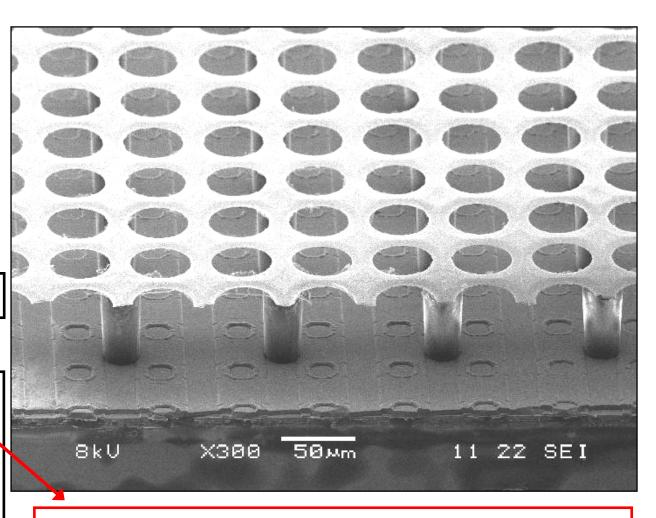
Now also Si<sub>3</sub>N<sub>4</sub> protection layers (7 μm<sub>2</sub>)
