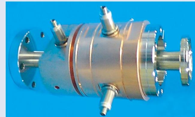
41 C and S-band Cavity BPMs, for use with Quad/Sext magnets with 100nm resolution (PAL, SLAC, KEK)
