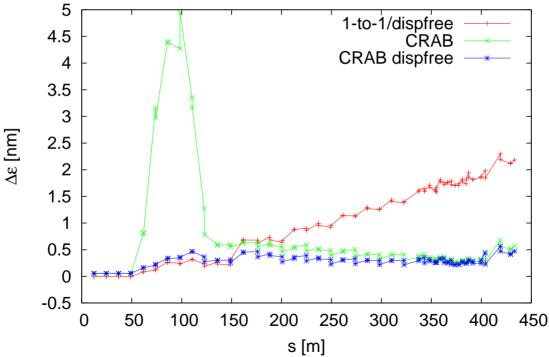
$\Rightarrow$  Final vertical emittance growth is 0.47 nm (it is 0.4 nm for Girder optimization)
