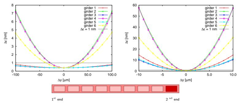
ullet Maximum allowed vertical displacement in  $\mu$ m that causes  $\Delta\epsilon_y \Rightarrow 1$  nm
