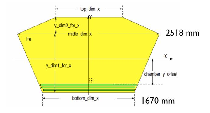
The ILD HCAL module: average x dimension ~ 2094 mm, corresponds to 70 cells of 30 x 30 mm<sup>2</sup>
