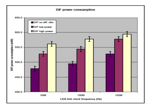
Power consumption vs. link frequency: relatively small power penalty from 50MHz=>150MHz
