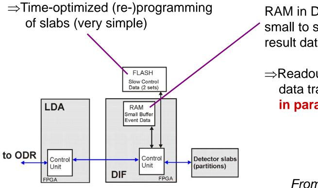
RAM in DIF FPGA is too small to store a full set of result data (slab readout)
