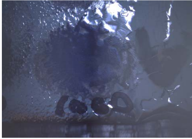
15min grind by polymond#1000 (10-20µm diamond)
