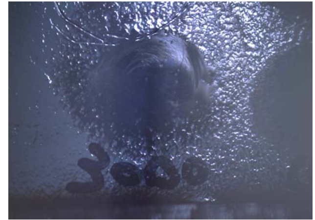
30min grind by polymond#3000 (3-8µm diamond)
