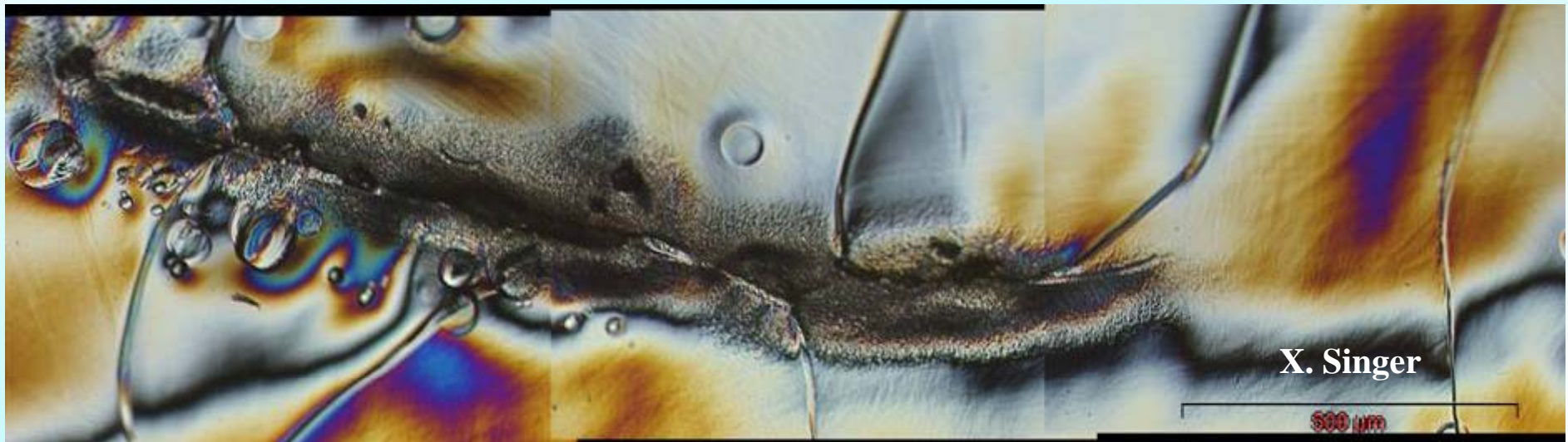
Light microscope. Quench location. Holes along grain boundaries. Cat's eyes.
